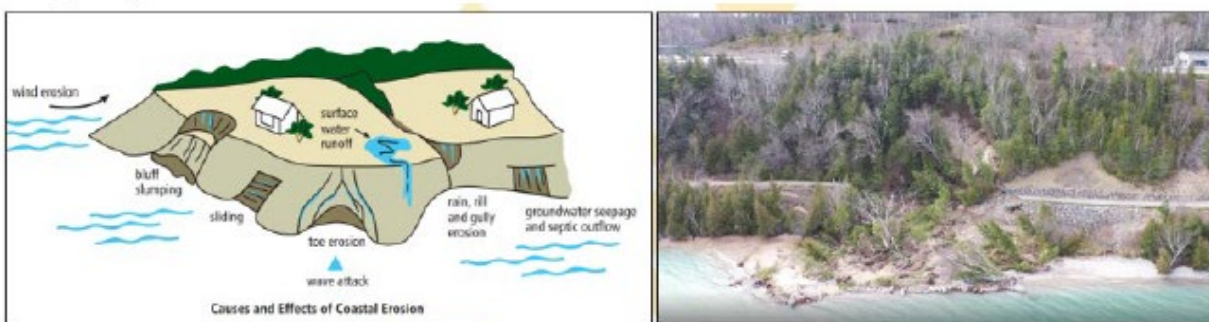
Figure 11: Slope Failure in Petoskev, MI
