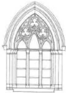
Figure 51: **Tracery:** Curvilinear openwork shapes of stone or wood creating a pattern within the upper part of a Gothic window; or an opening of similar character formed by the decorative treatment of mullions.
