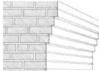
Figure 52: **Corbelling:** In masonry, a series of projections, each stepped progressively farther forward with height; anchored in a wall, story, column, or chimney; and used to support an overhanging member or ornament.
