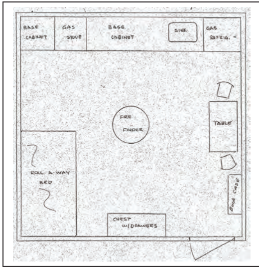
Fig. 16: Proposed layout of living space in new fire lookout tower cabs. Drawing by James Bowman, Park Engineer, in "Project Construction Proposal B-49-5, 1963." Image located in Record Group #79, Box 9, at Federal Records Center, Chicago, IL.
