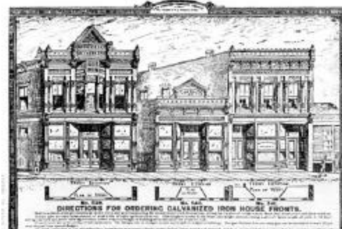
Figure 8: Trains brought stylish mail-order storefronts like this one to towns throughout Michigan. Arriving in town on Monday morning, the one-piece storefront could be swiftly assembled and operational before the week's end. Commercial property owners were important consumers of high style architecture.
