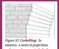
Figure 52: **Corbelling:** In masonry, a series of projections, each stepped progressively farther forward with height; anchored in a wall, story, column, or chimney; and used to support an overhanging member or ornament.
