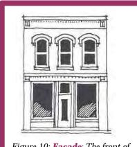
Figure 10: **Façade**: The front of a building; also any side of a building facing a public way or space.
