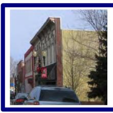
Figure 41: Most commercial structures have flat roofs hidden by the extension of the front wall plane.
