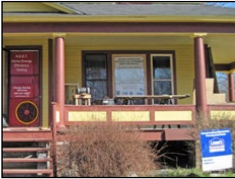
Blower door test house, Kalamazoo. CLG grant project. State Historic Preservation Office.
