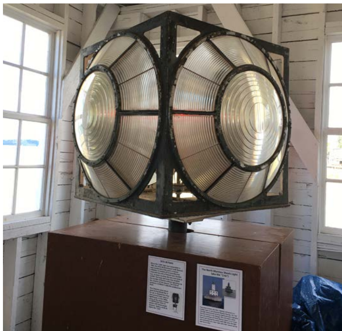
Figure 1C-01: Photo of the original 4-sided airway-beacon lens installed in the North Manitou Shoal Light Station from 1935 - 1980. This lens is currently on display at the Cannery Boat Museum in historic Glen Haven within the Sleeping Bear Dunes National Lakeshore.
