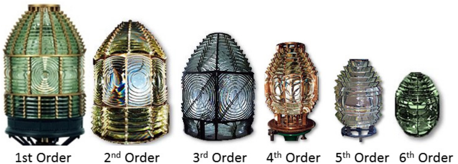
Figure 1A-04: Visual comparison of the six orders (sizes) of Fresnel lenses.
