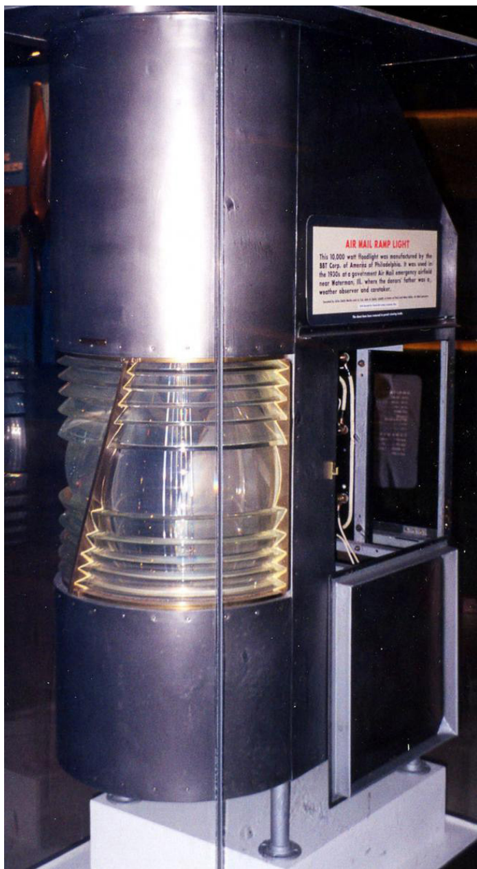
Figure 1A-05: Photo of a BBT Corp. of America (successor company of the French company Barbier, Bernard and Turenne that fabricated lighthouse Fresnel lenses) airport lens on display at the National Museum of the US Air Force Museum, Dayton, Ohio. This lens was used in the 1930s at a government Air Mail emergency airfield in Illinois.
