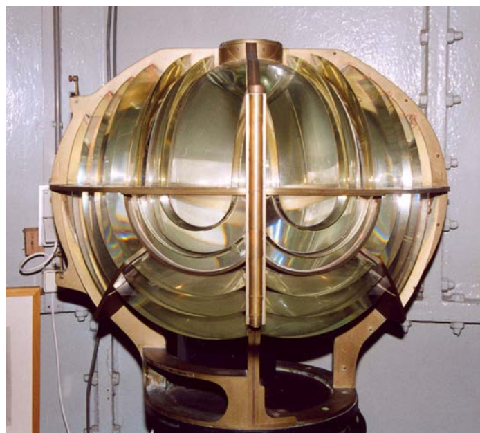
Figure 1A-06: Photo of a BBT Corp. of America Aviation Lens that gives a vertical shaft of light for aircraft navigation.
