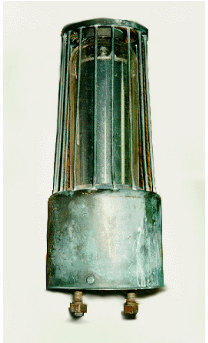
Figure 1A-10: Photo of a sun valve used in the earlier automation of lights. These flow control valves were used with acetylene illumination systems prior to electricity. The valve is controlled by four metal rods enclosed in a glass tube. The central rod that is blackened is surrounded by the three polished rods. As sunlight falls onto all of the rods, the absorbed heat of the sun allows the unequally expanding dark rod to cut the acetylene gas supply. After sunset, the central rod cools down, becoming the same length as the polished rods and opening the gas supply.
