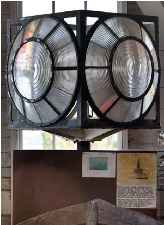
Figure 1A-07: Photo of the 4-sided airway-beacon lens originally installed in the North Manitou Shoal Light Station in 1935. This lens was removed in 1980 and is currently on display at the Cannery Boat Museum in historic Glen Haven within the Sleeping Bear Dunes National Lakeshore.
