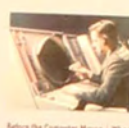
Before the Computer Wars | When SAGE operators wanted to identify a flight on the display screen, they pointed a light gun at the spot and pushed the target flight identification wheel that appeared on the screen.
