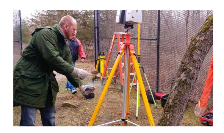
Simply put, LiDAR uses pulses of light (harmless lasers) to detect and measure the three-dimensional (3D) world. LiDAR instruments can be mounted on a tripod, on a vehicle, or on a manned aircraft or unmanned drone. LiDAR
